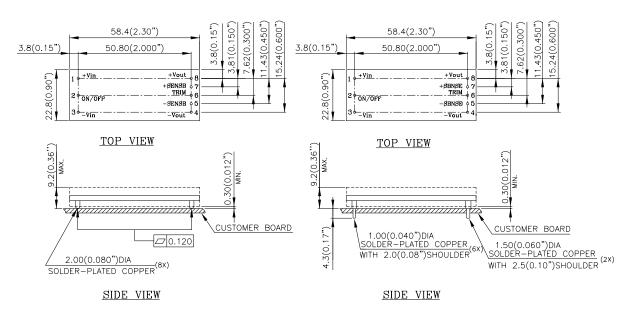
DIMENSIONS ARE IN MILLIMETERS AND (INCHES) TOLERANCES: X.Xmm±0.5mm(X.XX in.±0.02 in.) X.XXmm±0.25mm(X.XXX in.±0.010 in.)
