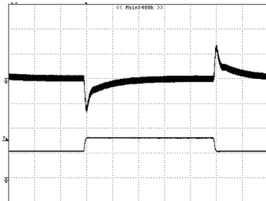
Figure 8: Output voltage response to step-change in load current (75%-50%-75% of I_{o, max} ; di/dt = 0.1A/\mu s ). Load cap: 10 \mu F tantalum capacitor and 1 \mu F ceramic capacitor. Top Trace: V_{out} (200mV/div, 200 \mu s /div), Bottom Trace: I_{out} (2A/div). Scope measurement should be made using a BNC cable (length shorter than 20 inches). Position the load between 51 mm to 76 mm (2 inches to 3 inches) from the module
