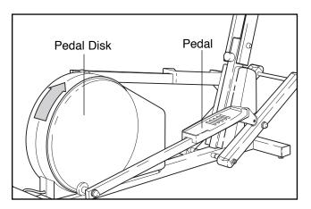
To dismount the elliptical crosstrainer, wait until the pedals come to a complete stop. **CAUTION: The elliptical crosstrainer does not have a freewheel; the pedals will continue to move until the flywheel stops.** When the pedals are stationary, step off the highest pedal first. Then, step off the lowest pedal.
