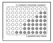
segment. The setting of the first segment is shown in the flashing CURRENT SEGMENT column of the LED matrix. The settings of the next seven segments are shown in the columns to the right. When only three seconds remain in the first segment, three tones will sound. All settings will then move one column to the left. The setting of the second segment will then be shown in the CUR-RENT SEGMENT column and the elliptical crosstrainer will adjust to the second setting.
