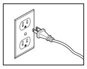
Note: To decrease the possibility of damaging your machine, always use a surge protector. Each time the power cord is plugged in, the incline frame will move to the lowest position. In addition, the incline frame may automatically move up and down as the elliptical crosstrainer goes through a calibration sequence.
